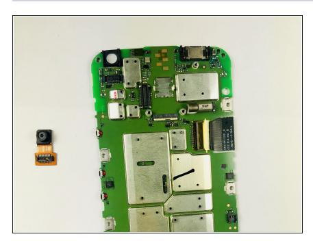
Remove the front camera from the device.
