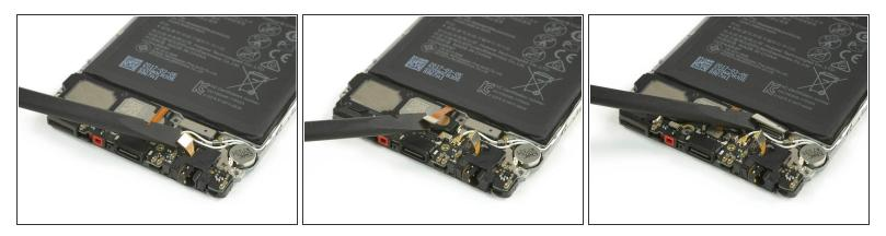
Use a spudger to disconnect the headphone jack flex cable, the loudspeaker flex cable and the main flex cable.
