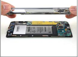
Press down on the back of the battery while you lift up on the edges of the midframe to separate the midframe from the rest of the phone.
