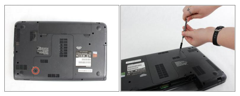
Remove one screw with a JIS #000 screwdriver.
