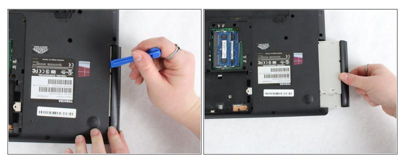
• Using a plastic opening tool, pry open the disk drive. Once it has loosened it will pull out.
