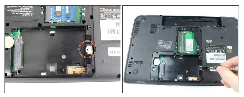
Remove a .5mm screw with a JIS #000 screwdriver.
