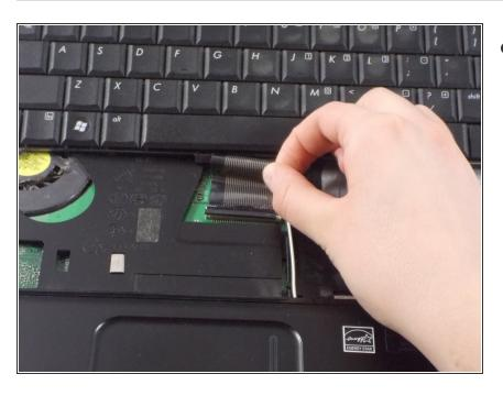
Carefully unclip and remove the large black wire that is connecting the keyboard to the laptop
