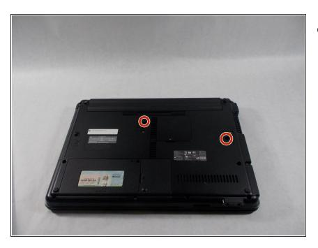
Turn the laptop over, the screws for the keyboard are in the middle and left of the device
