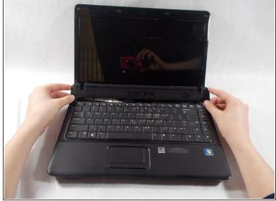
Gently use a plastic spudger to remove the plastic holder at the top of the keyboard
