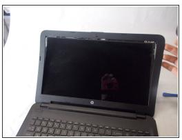
Carefully use the blue plastic opening tool to remove the outer frame of the screen.
