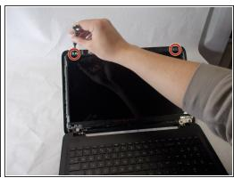
• Using the Phillips #0 screwdriver, unscrew the 4 screws around the frame.
