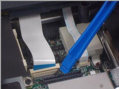
• Use a plastic opening tool to disconnect both cable connectors gently.
