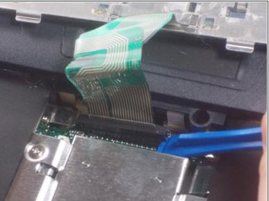
Disconnect the green ribbon cable using a plastic opening tool.
