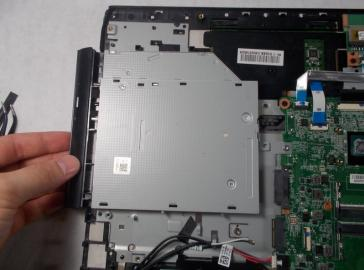
• Gently pull the CD drive out, disconnecting it from the motherboard connector marked in blue.
