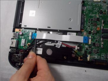
• Remove the ribbon by flipping up the tabs and using the black tweezers to gently pull the ribbon out from both ends.
