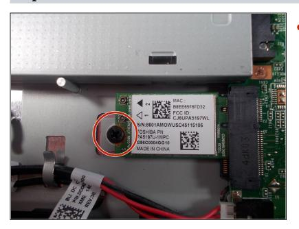
Remove the 3mm Phillips head screw with a Phillips #00 screwdriver.
