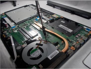
• Unscrew the two 3mm Phillips head screws on each fan using the Phillips #00 screwdriver.
