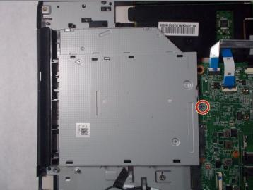
• Remove the 3 mm Philips head screw that connects the CD drive to motherboard with a Phillips #00 screwdriver.
