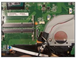
• Remove the wires from the motherboard using the tweezers.
