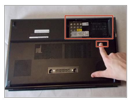
Slide the lock key to unlock the battery. Then you can lift the battery from its holder.
