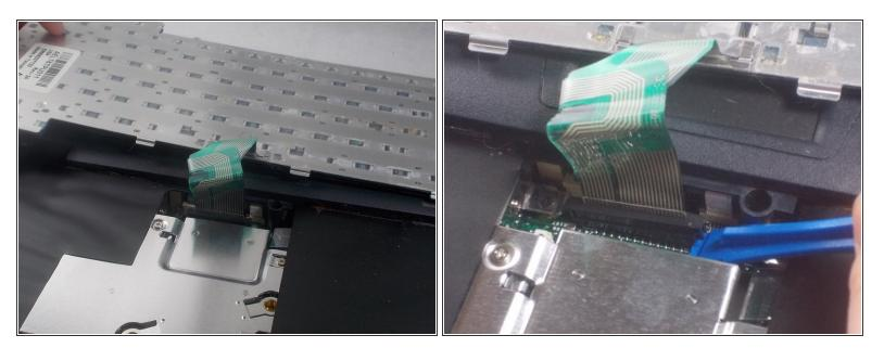
• Disconnect the green ribbon cable using a plastic opening tool.
