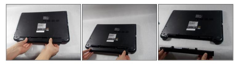
• Once the screws are removed, slide the battery pack out of the computer.
