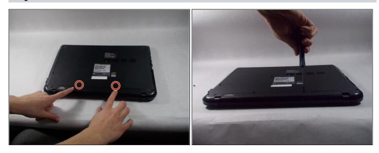
• Remove the two 6.5 mm Phillips head screws indicated using a Phillips #00 screw driver.
