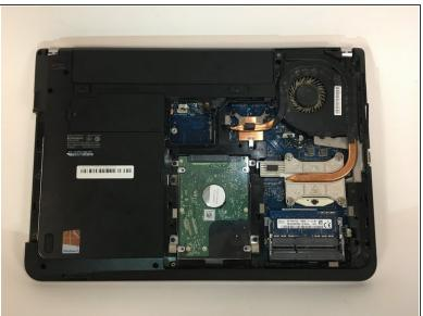
Remove the back panel of the device.
