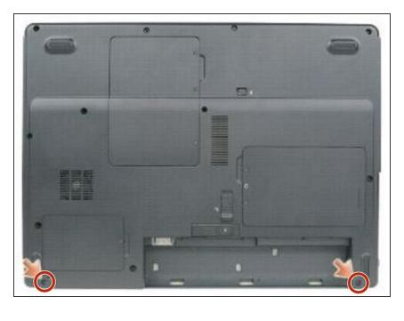
From the bottom of the computer, remove the two M2.5 x 8-mm screws labeled "D."
