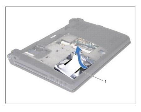
Tilt the hard drive by 45-degrees and lift it out of the computer base.
