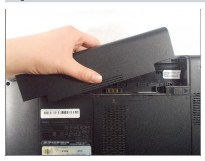
Pull battery away from computer until it is fully removed.
