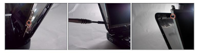
Unscrew the four 2x3 mm screws from the two sides on both the top and bottom.
