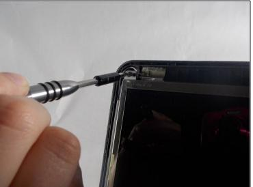
• Unscrew the two 2.5x4 mm screws from the top of the screen.
