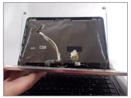
• The screen can now be fully removed from the computer.
