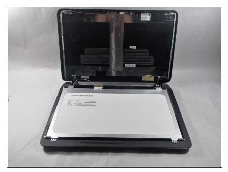
Remove the screen and place the screen very softly on the keyboard.
