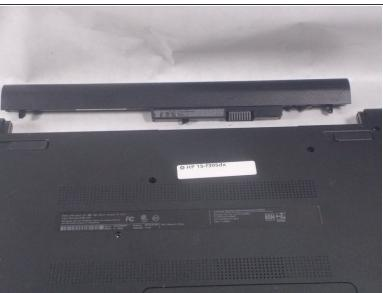
• Lift the battery from the middle and then pivot it outward to remove it from the computer.
