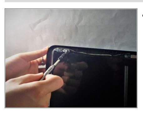
Remove the four 3mm PH1 Phillips head screws in each corner of the screen and do not care about outer screws.
