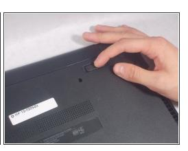
Firmly slide the release latch to unlock the battery and slide the battery release latch to release the battery.
