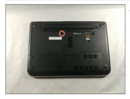
• Remove the single screw that secures the cd drive to the laptop noted by the red circle
