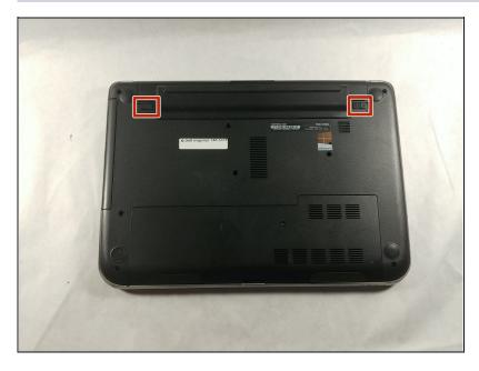
Push the two sliders away from the battery towards the outer edges.
