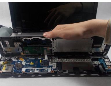
Use a metal spudger to lift up and pull back the track pad
