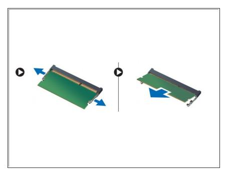
Pry the securing clips away from the memory module until it pops-up and remove the memory module from its connector on the system board.
