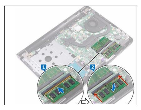
Slide the **NEW** memory module firmly into the slot at an angle and press the memory module down until it clicks into place.
