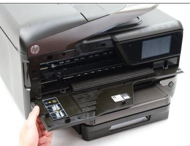
Open the front panel door by pulling forward on the slot located on the front-left side of the printer.
