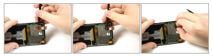
• Pry up the camera's connector to the motherboard with the nylon spudger.
