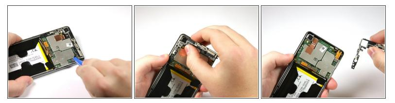
• Pry up the black camera case with the plastic opening tool and then remove the case.
