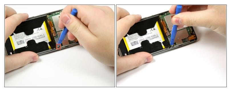
• Pop off the small connector on the right side of the motherboard with the plastic opening tool.
