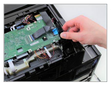
Remove the black brace from the right side of the motherboard, located near the black ribbon cable.
