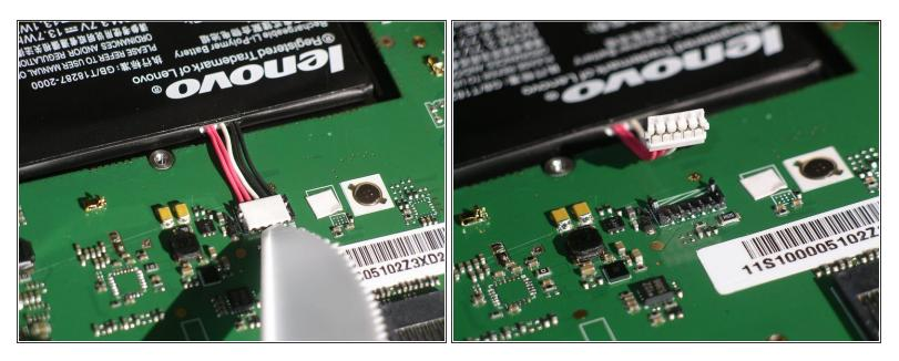
• With the glue loose, and the wires removed, the battery is available as a spare for me.
