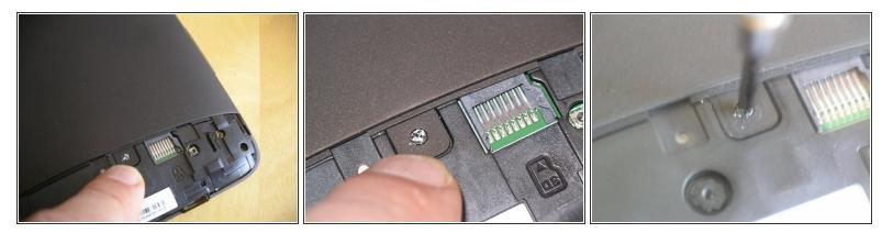
• The rear cover wouldn't pull off, even when prying with my "spudger". I didn't want to break the tablet (yet). Then I noticed the round white spot. I scraped away the brittle white paint, exposing another phillips screw, and removed it. (There goes my warranty! They made it tamper evident.)
