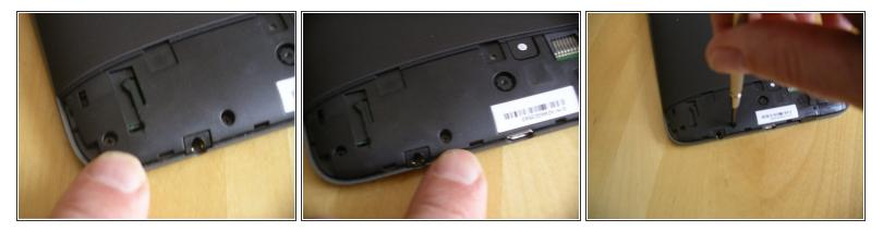
• A number 0 phillips screw driver works for all of these screws, and all steps going forward.
