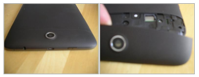
We're looking at the rear top here. It just slides toward the top of the tablet and lifts off, exposing the camera and micro SD card holder.
