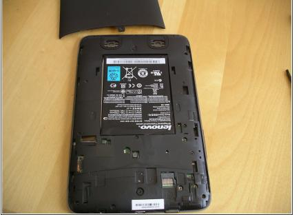
Stero speakers are at the tablet's bottom. The 3.7 VDC Lithium Polymer battery is right there. 13.7 Wh / 3700 mAh. Fairly large for a cheap tablet. It adds to the heft of this tablet.
