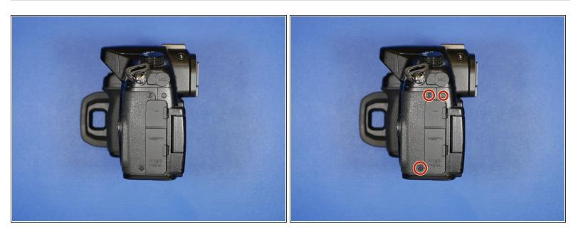
• Remove the three screws on the left hand side of the camera.
