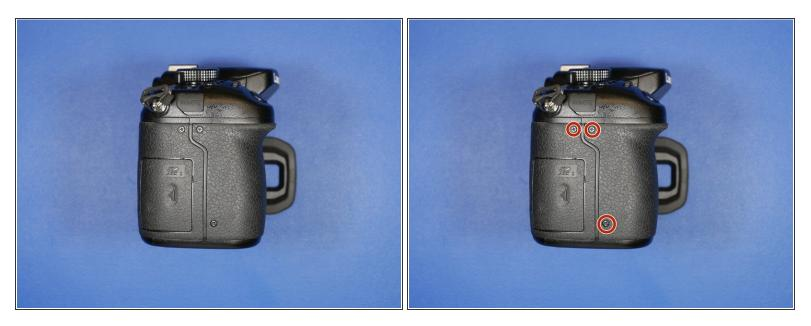
• Remove the 3 screws on the right hand side.
