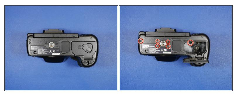
• There are 6 screws on the bottom of the camera. One is hidden in the battery compartment.
