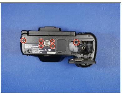
There are 6 screws on the bottom of the camera. One is hidden in the battery compartment.
