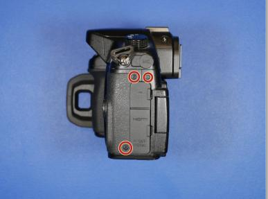
Remove the three screws on the left hand side of the camera.
