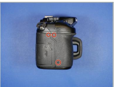
Remove the 3 screws on the right hand side.
