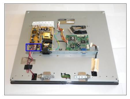
Disconnect the two connectors to the speakers by gently pulling on the hard plastic straight up.
