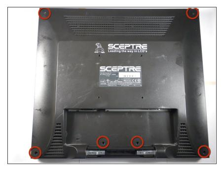
Using a #2 Phillips screwdriver, remove the six 7mm screws at the circled locations.
