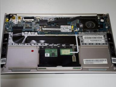
Lift the battery directly up and remove it from the device.
