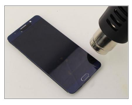
Heat the display for two minutes with a heat gun.
