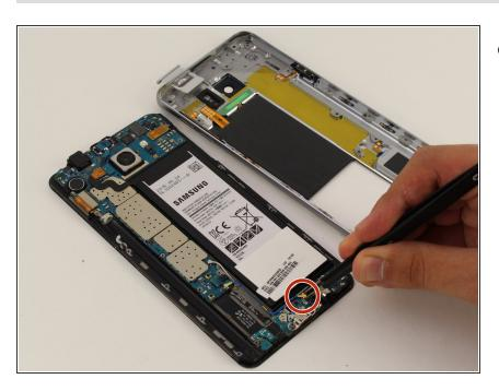
Loosen the two signal cable connectors.
