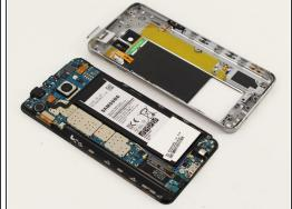
Grip the back of the device and press down on the white square to remove the middle housing.
