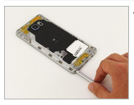
Remove the S-Pen from the bottom of the device.
