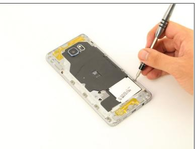
Remove 20 5mm screws with a Phillips #1 Screwdriver.
