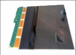
• Lift the LCD back cover to reveal the LCD screen below.
