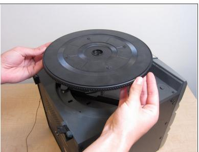
Separate the turntable from the top of the record player by lifting straight up.
