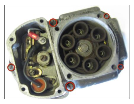
Use a #2 Flathead screw driver to remove the five screws on the body of the magneto, indicated by the red circles.
