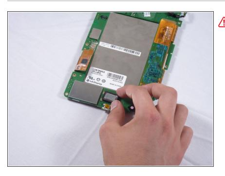
Mhen replacing the motherboard make sure that the speaker assembly component (small rectangular piece) is in place. It is not attached and needs to be properly aligned.
