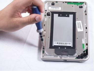
Remove the ten T5 screws from around the edges of the silver midframe.
