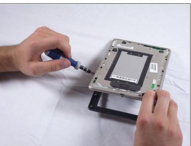
Using a spudger or plastic opening tool, carefully pry the screen bezel away from the silver midframe.
