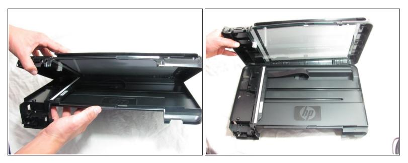
• Lift the scanning lid from the lower portion of the printer hood.
