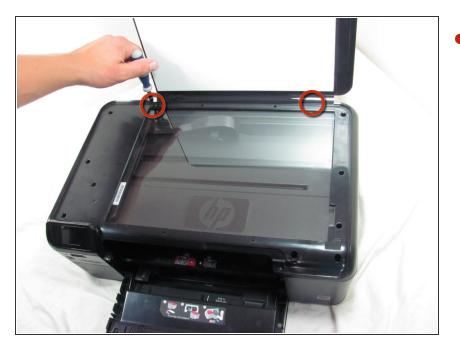
• Use a T10 screwdriver to unscrew the two screws that fasten the frame to the printer hood.
