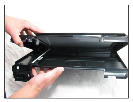
• Pull the printer hood upward.
