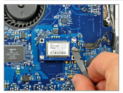
Use the flat end of a spudger to pry the Bluetooth antenna cable connector up off the Bluetooth board.
