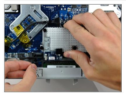
De-route the speaker cables from beneath the IR Board and heatsink assembly.
