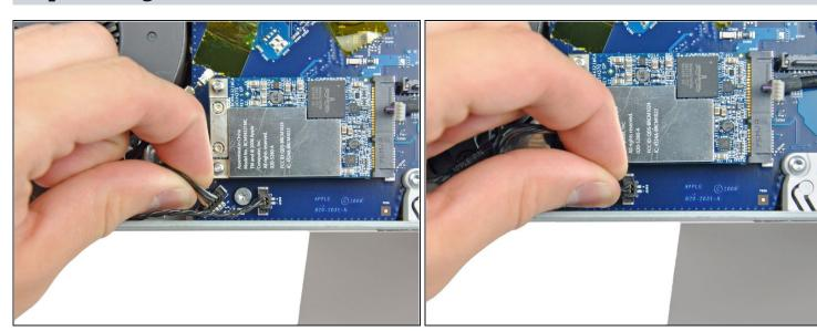
• Disconnect the HDD fan and power button from the logic board by pulling their connectors straight up off the sockets on the logic board.
