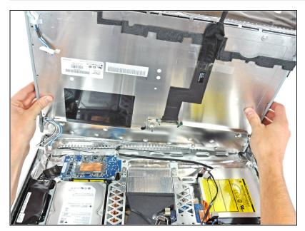
Rotate the display until it is nearly perpendicular to the rear case and lift it up to peel it off the EMI shield stuck to its top edge.
