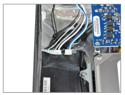
Disconnect the two inverter cables at the top edge of the inverter using the method explained in the previous step.
