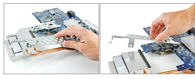
Carefully lift both metal heat sink brackets off the logic board.
