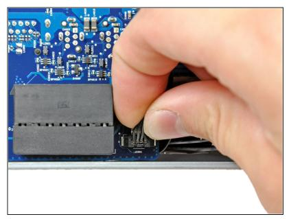
Pull the ambient light sensor cable connector up off the logic board.
