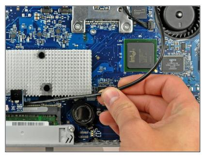
Carefully de-route the IR board cable out from under the IR board and move it out of the way of the logic board.
