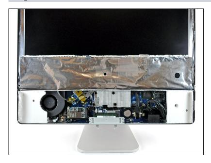
Tape the EMI shield to the face of the display to keep it out of the way.
