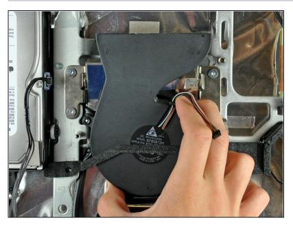
Pull the CPU fan off the plastic posts protruding from the rear case and remove it from the iMac, minding any cables that may get caught.
