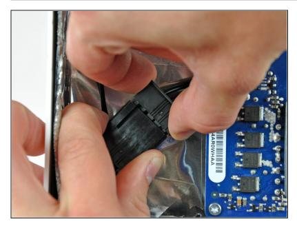
Disconnect the inverter cable by pulling the connector away from its socket.
