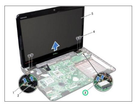
Route the Mini-Card antenna cables and display cable through the routing guides.
