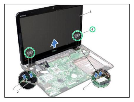
Hold the display assembly in place and remove the four screws that secure the display assembly to the computer base.
