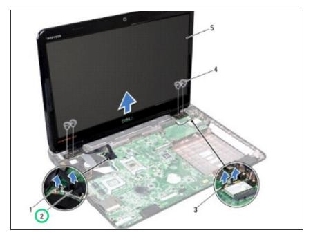
Connect the display cable to the connector on the system board, and replace the display cable grounding screw.
