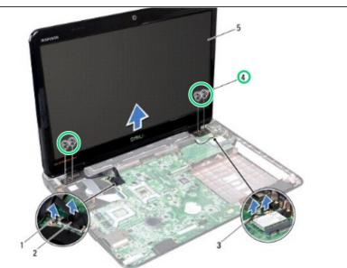
Place the NEW display assembly in position and replace the four screws (two on each side) that secure the display assembly to the computer base.
