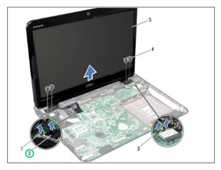
Disconnect the display cable from the connector on the system board, and remove the display cable grounding screw.
