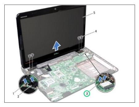
Make a note of the Mini-Card antenna cables and display cable routing and remove the cables from the routing guides.
