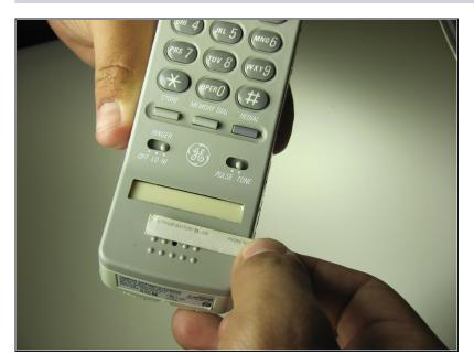
Remove the paper with a plastic opening tool by gently sliding the tool underneath and prying the paper away from the phone.
