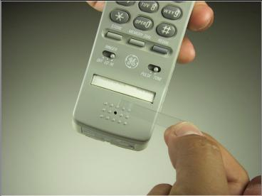
Remove the plastic cover with a plastic opening tool by gently sliding the tool underneath the plastic and pry the cover off.
