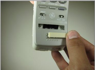
Remove the rubber stopper with a plastic opening tool by gently sliding the tool underneath and pry away from the phone.
