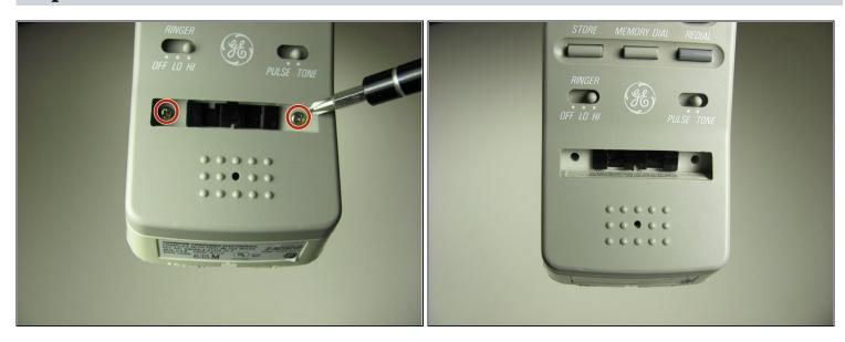
• Remove the two 2.1 mm screws with a Phillips #1 screwdriver.
