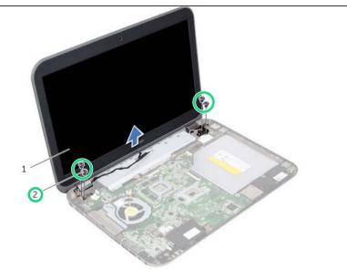
Place the display assembly in position and replace the screws that secure the display assembly to the computer base.
