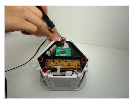
Unscrew all visible of the screws on the black logic board cover with the larger screwdriver.
