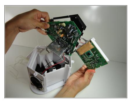
• Flip the screen and the logic board over to the right side.
