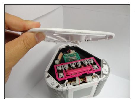
• Take off top piece by using slight force and pulling off.
