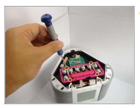
• Unscrew the button board with smaller screwdriver.
