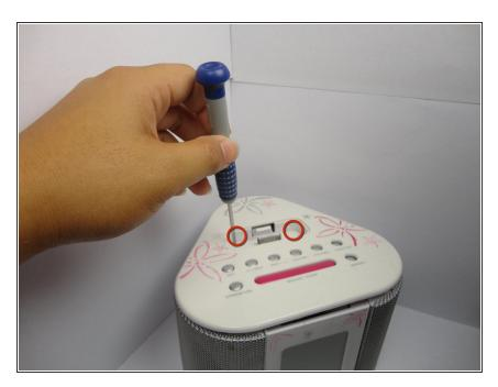
• Unscrew the 2 screws on the top of the device, next to the docking plug.
