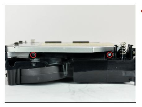
Turn the mini 180 degrees and remove the two Phillips screws securing the optical drive to the internal frame on the other side.
