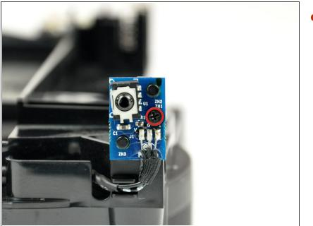
Remove the single Phillips screw securing the IR board to the internal frame.
