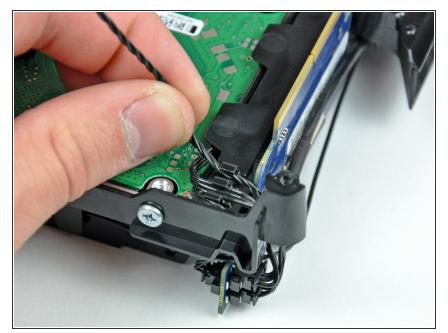
• De-route the IR board and cable through the small plastic clip in the internal frame.
