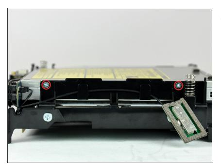
Remove the two Phillips screws securing the optical drive to the internal frame.
