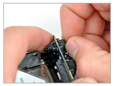
Use your fingers to disconnect the IR cable connector from its socket on the interconnect board. Make sure to pull straight out, and to pull on the connector and not the cable.
