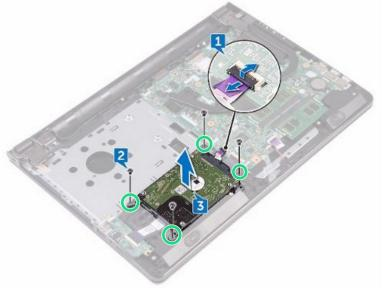
• Place the hard-drive assembly in the palm-rest assembly and align the screw holes on the hard-drive assembly with the screw holes on the palm-rest assembly.
