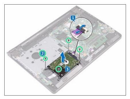
Replace the four screws (M2x3) that secure the hard-drive assembly to the palm-rest assembly.
