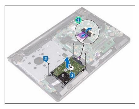
Slide the hard-drive cable into its connector on the system board and close the latch to secure the cable.
