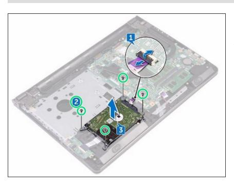
Remove the four screws (M2x3) that secure the hard-drive assembly to the palm-rest assembly.
