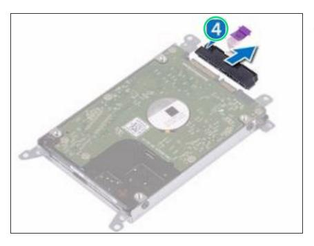
Disconnect the interposer from the hard-drive assembly.
