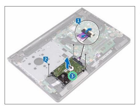
Lift the hard-drive assembly off the palm-rest assembly.
