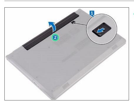
Using your fingertips, lift the battery at an angle and remove it from the battery bay.
