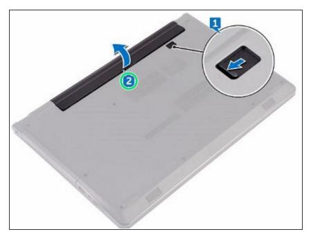
Place the battery in the battery bay and snap the **NEW** battery into place.
