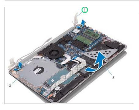
Using the alignment posts, press the display hinges down on the palm rest and keyboard assembly.
