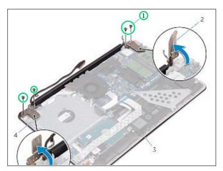
Replace the screws that secure the display hinges to the palm rest and keyboard assembly.
