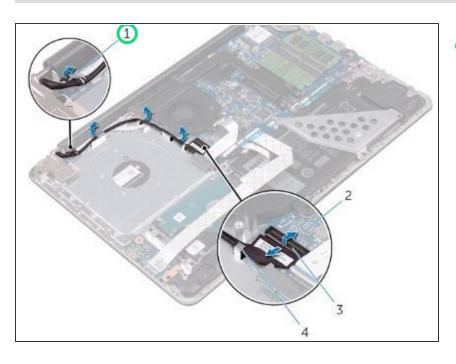
Route the display cable through the routing guides on the palm rest and keyboard.
