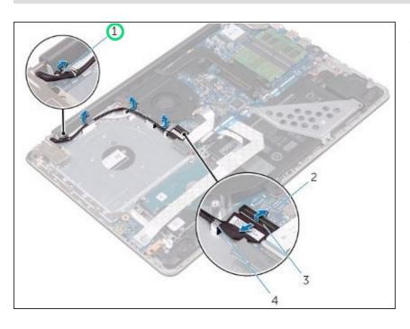
Note the display cable routing and remove the cable from its routing guides.
