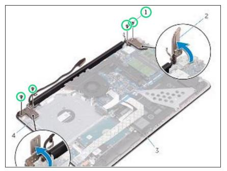
Remove the screws that secure the display hinges to the palm rest and keyboard assembly.
