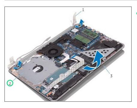
Lift the palm rest and keyboard assembly off the display assembly.
