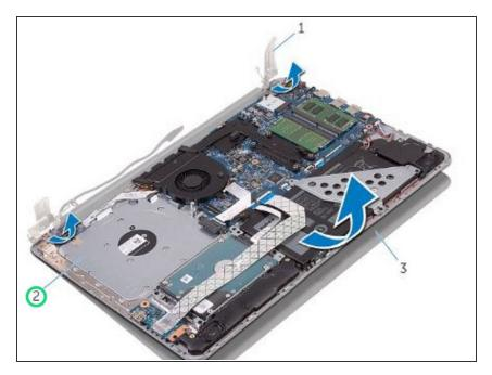
Place the palm rest and keyboard assembly on the NEW display assembly.
