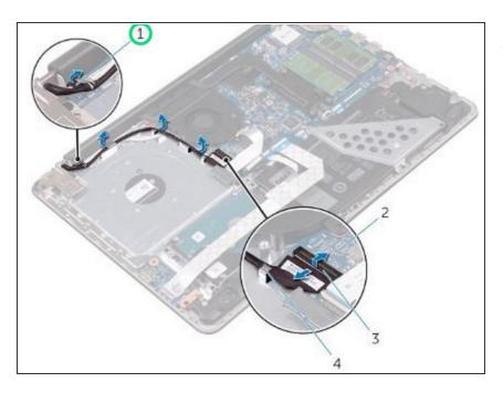
Slide the display cable to the connector on the system board and close the latch to secure the cable.
