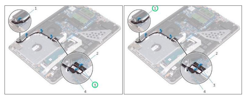
Lift the latch and disconnect the display cable from the system board.
