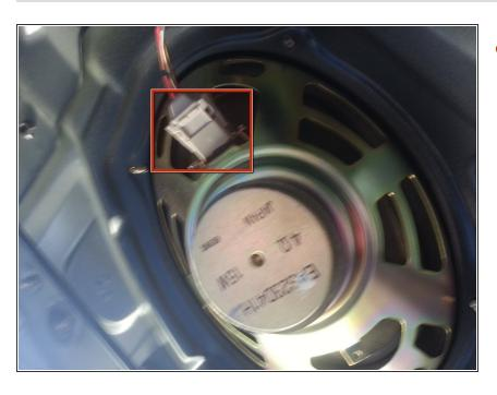
Disconnect the wiring harness in trunk.
