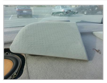
Slide the speaker panel towards the center of car and pull it out.
