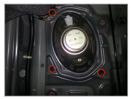
Remove the three screws holding the speaker panel in place.
