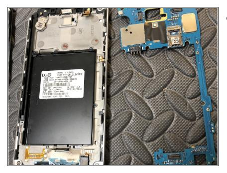
With the flex cables detached, remove the motherboard from the frame. Be careful as there is a small lip that inserts under the rear camera bracket. Easiest to loosen from the bottom and then lift the part near the volume button and lightly pull to the right and then up.
