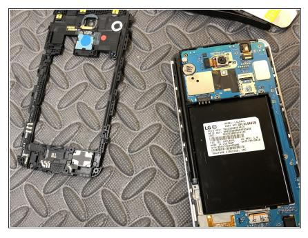
Use your fingers or a flat pry tool and remove the plastic shield from the outer. If you use a flat pry tool be careful not to insert to far as it may cause damage. This will expose the motherboard.
