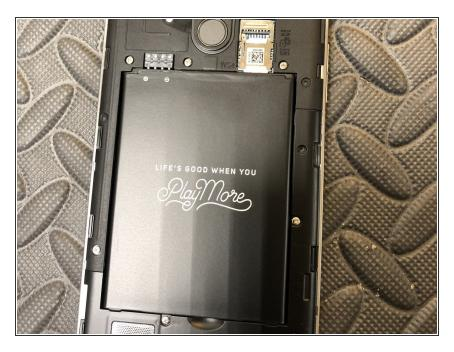
With the rear cover removed, now remove the battery from the casing.
