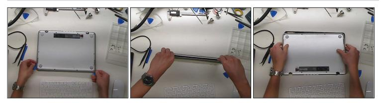
Use a plastic pry tool to get in-between the bottom cover and the lower case assembly.
