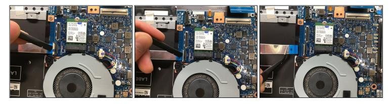
• Use the tip of a spudger to flip up the retaining flap on the daughterboard ribbon cable ZIF socket on the motherboard.
