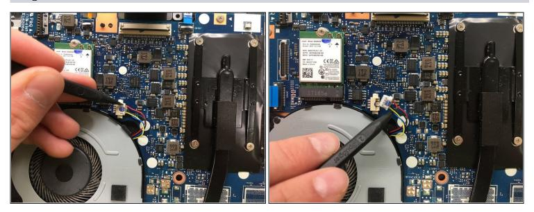
• Use the tip of spudger to push out the fan connector.
