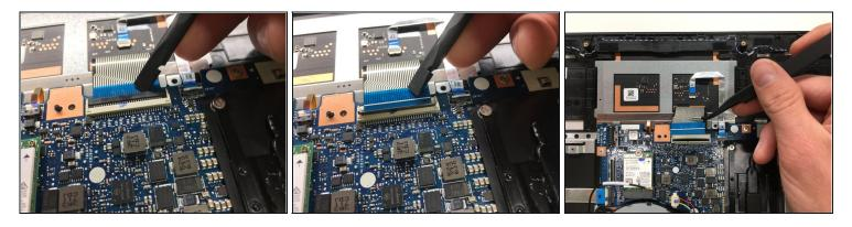
• Use the tip of a spudger to flip cup the retaining flap on the keyboard ribbon cable ZIF socket.
