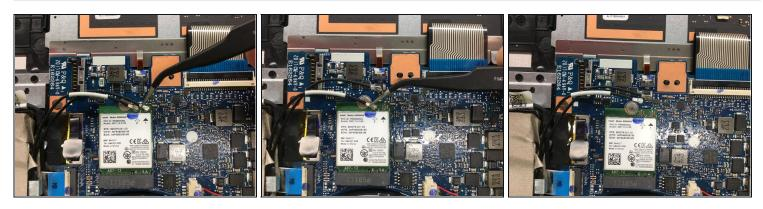
Disconnect the Wifi/Bluetooth RF cables from the wireless card.
