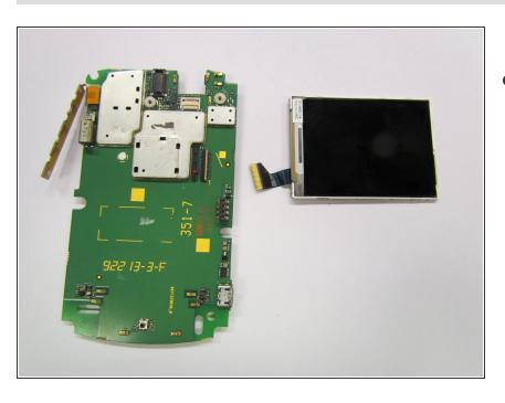
Insert the new LCD screen into the circuit.
