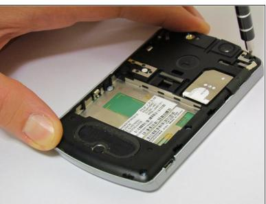
Remove the 6 screws using the T5 torx screwdriver.
