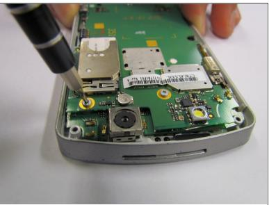
Remove both screws on the mounted surface with a T5 screwdriver.
