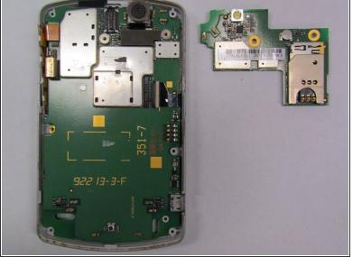
Remove the glued, mounted surface by lifting it from underneath the SIM card slot by using the plastic opening tool.
