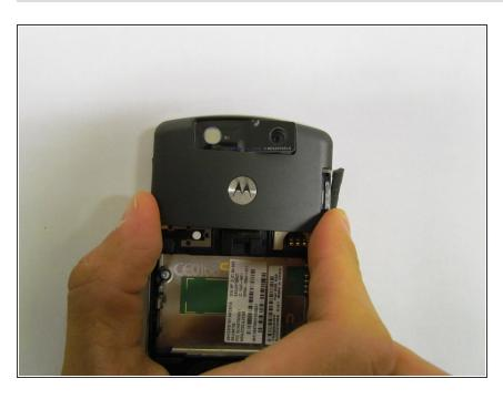
Press inwardly on the upper casing to release.
