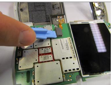
Lift the motherboard about 90 degrees and remove the circuit with the orange ribbon (from the keyboard) by gently lifting the circuit.
