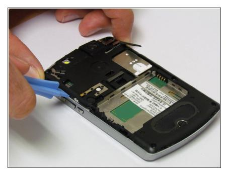
Once the screws are removed, use the plastic opening tool to remove the black casing.
