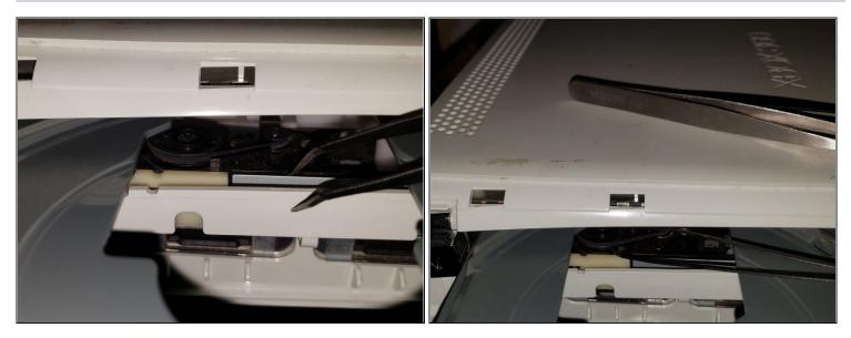
• Use <u>tweezers</u> to take a rubber belt of 2 pulleys in between the hole in the DVD Tray.
